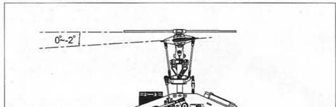
Stick position at low/Throttle 0%/Pitch0~-2° 搖桿低速/油門0%/Pitch0~-2°
