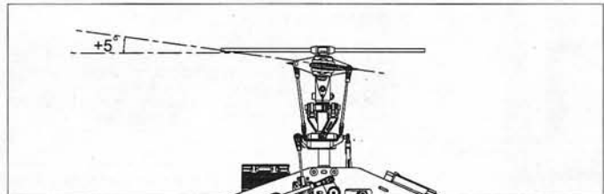
Stick position at Hovering/Throttle 70%/Pitch+5° 搖桿停懸/油門70%/Pitch+5°
